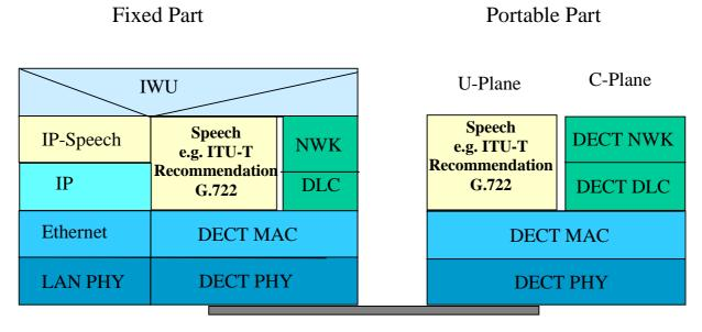
Figure 11: Protocol architecture for transport of speech
