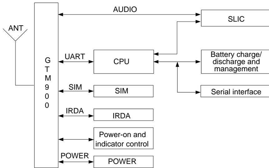
**Figure 1-3** Functional architecture of terminal-type fixed station
