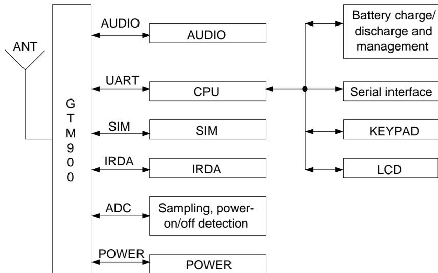
**Figure 1-4** Functional architecture of phone-type fixed station
