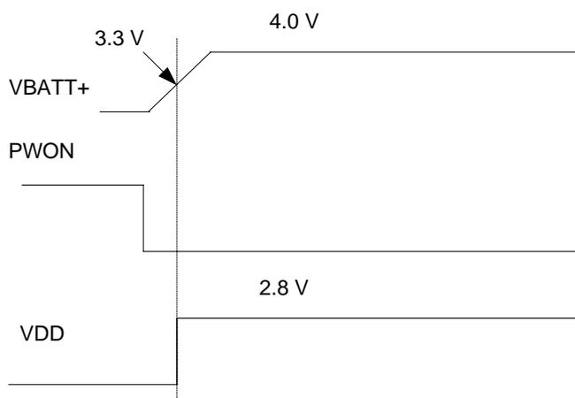
**Figure 5-1** Relationship between VDD and PWON signal
