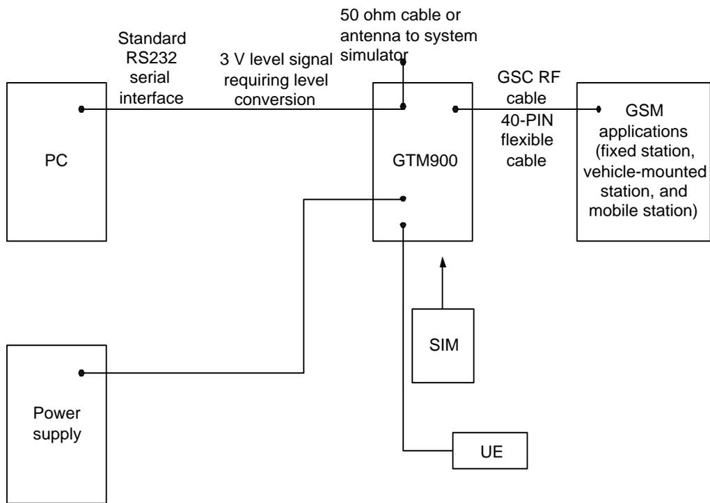
**Figure 5-3** Functionality of GTM900
