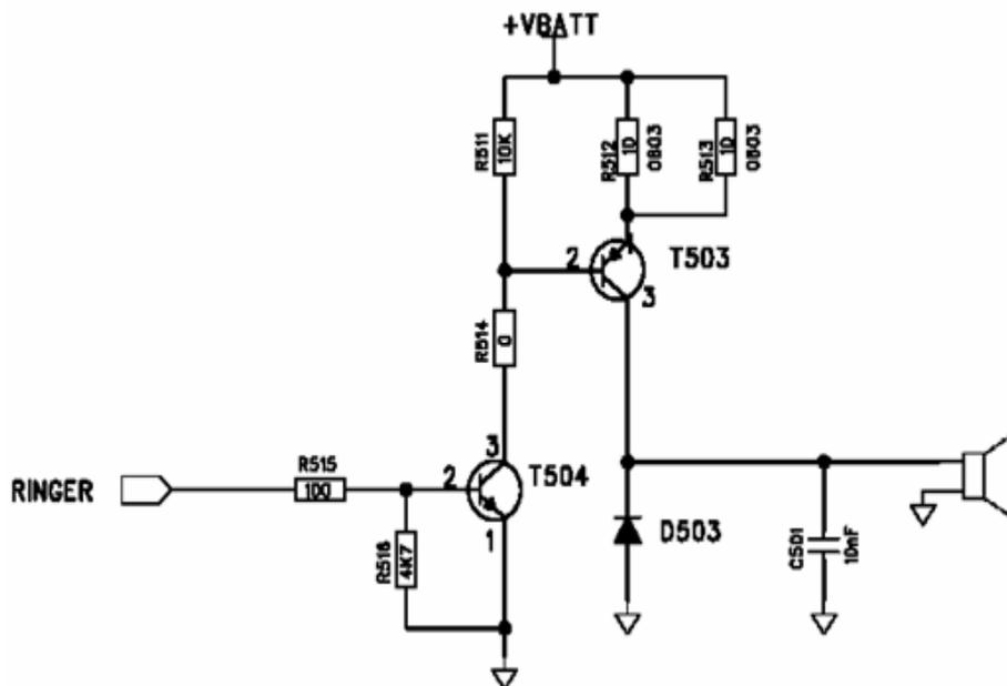
**Figure 4-3** Drive circuit of Ringer signals
