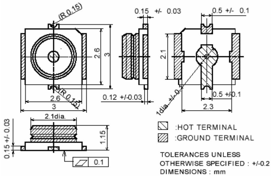
Figure 2-2 Dimensions of antenna connector (unit: mm)
