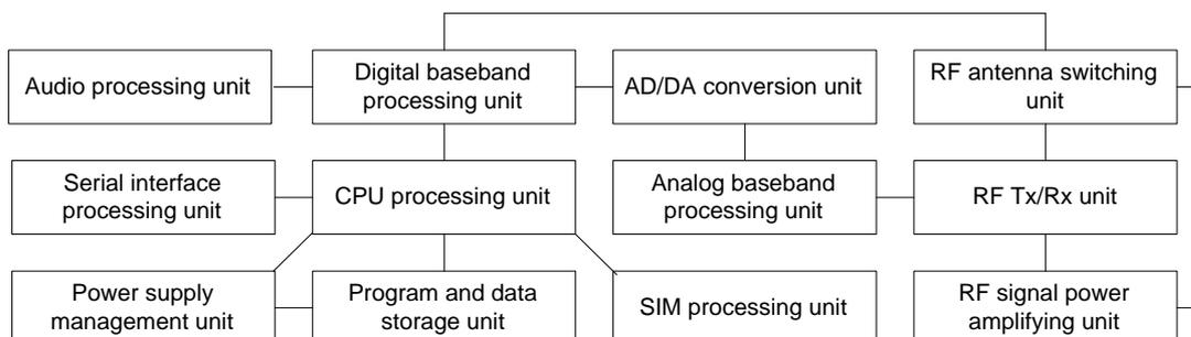
**Figure 1-2** Functional architecture of GTM900
