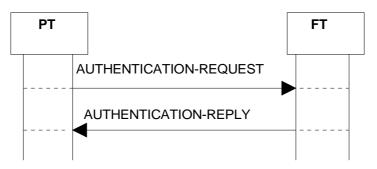
NOTE: If the received RES value in the {AUTHENTICATION REPLY} message is not equal to XRES1 further actions taken by the PT depend on the PP application.
