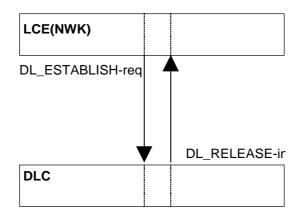
Figure 74: Direct PT initiated link establishment failure
