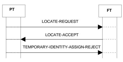
Figure 55: Rejection of identity assignment
