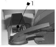
Step7: Connect one of the two SPIRAL CABLE plugs E to Jack 2.
