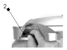
Step 8: Connect the other SPIRAL CABLE E plug to the handset Jack.
