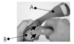
Steps 2-3: Lock the group (BRACKET B + HANDSET A) to the BASE C.
