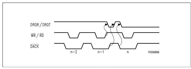
Figure 45 DMA-Transfers with Pulsed DACK (read or write)
