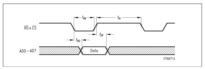
Figure 103 Microprocessor Read Cycle
