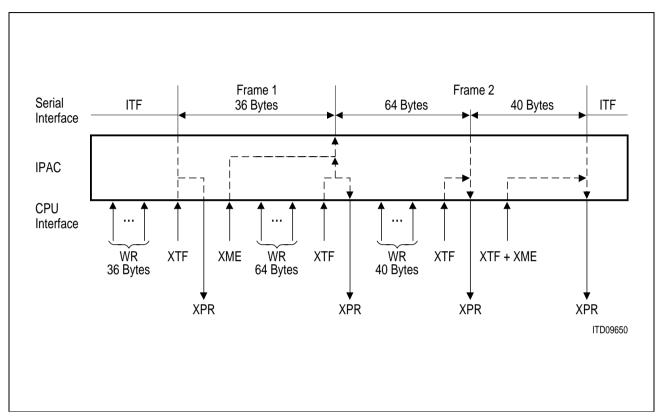
Figure 83 Continuous Frames Transmission Sequence Example
