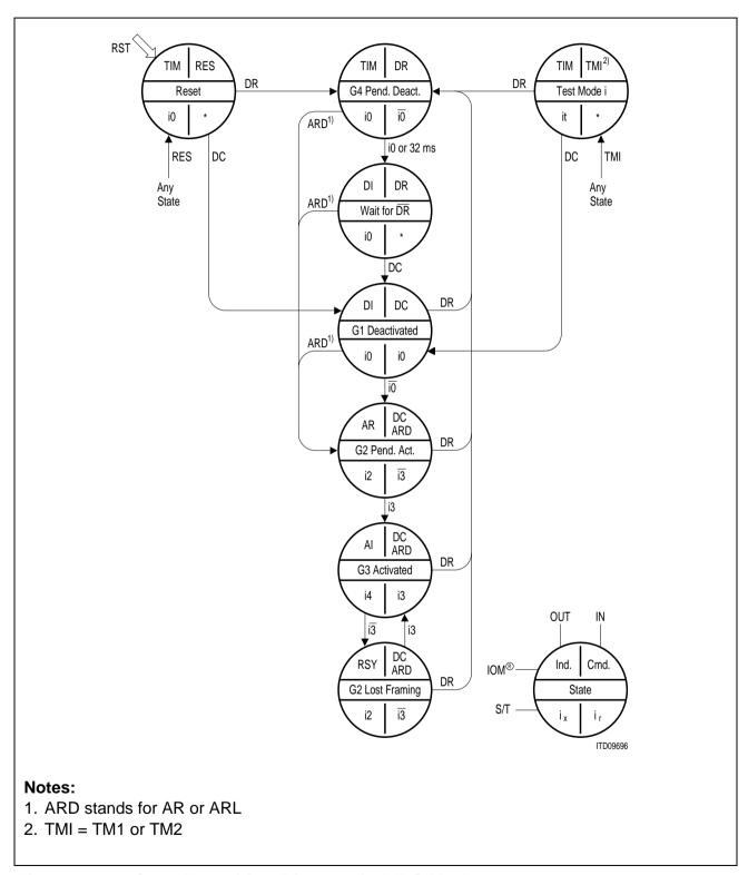
Figure 121 State Transition Diagram in LT-S Mode
