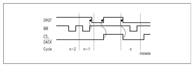
Figure 41 Timing Diagram for DMA-Transfers (slow) Transmit (n < 64, remainder of a long message or n =  $k \times 64$ )
