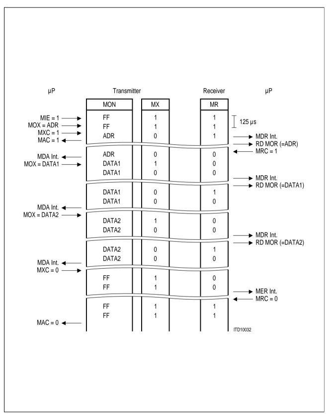
Figure 63 MONITOR Channel Protocol (IOM®-2)
