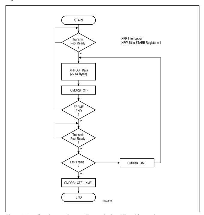
Figure 82 Continuous Frames Transmission (Flow Diagram)
