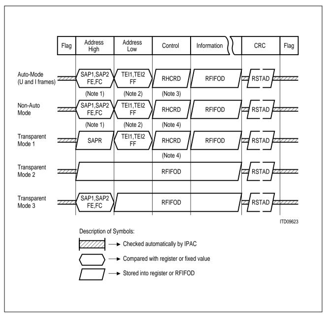
Figure 15 Receive Data Flow
