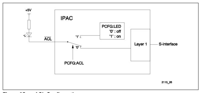
Figure 35 ACL Configuration
