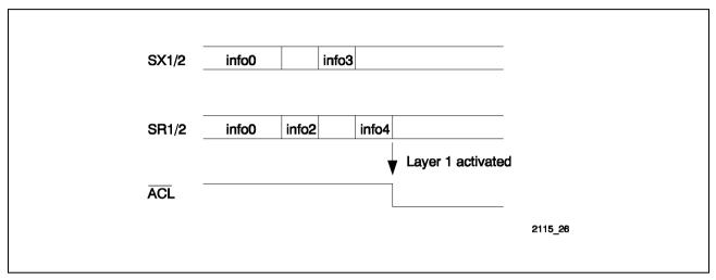
Figure 34 ACL Indication of Activated Layer 1
