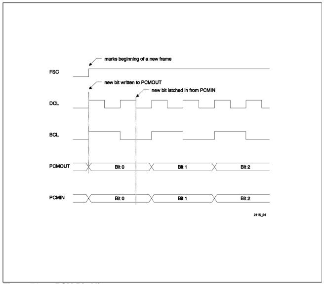
Figure 71 PCM Bit Alignment
