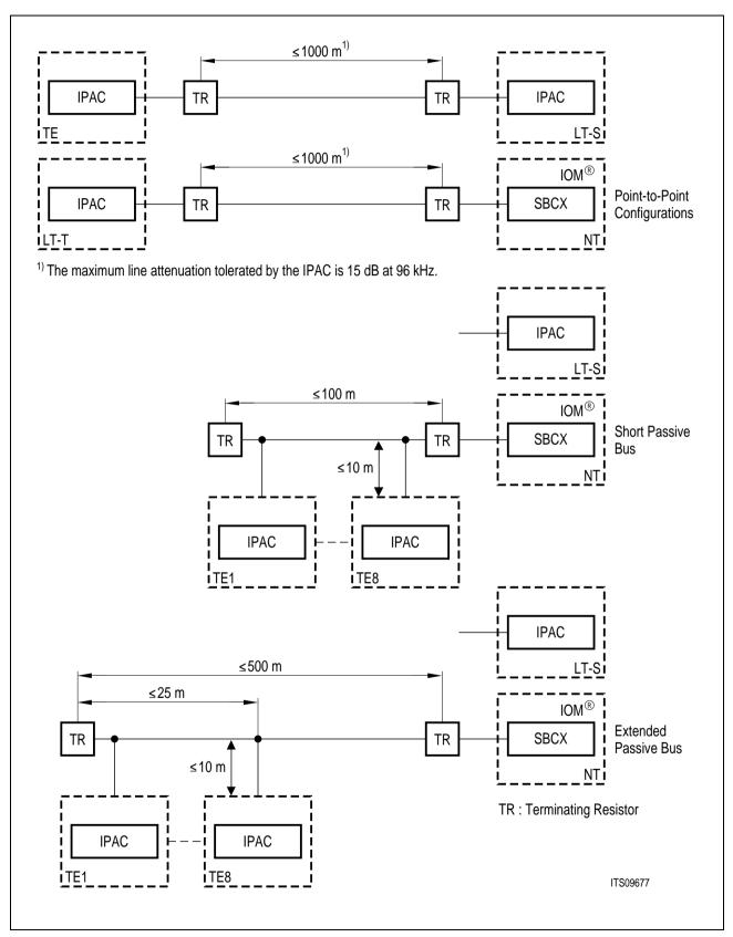
Figure 24 Wiring Configurations in User Premises
