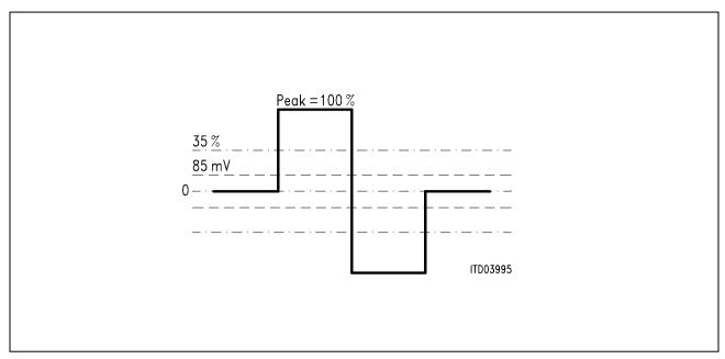
Figure 30 Receiver Thresholds
