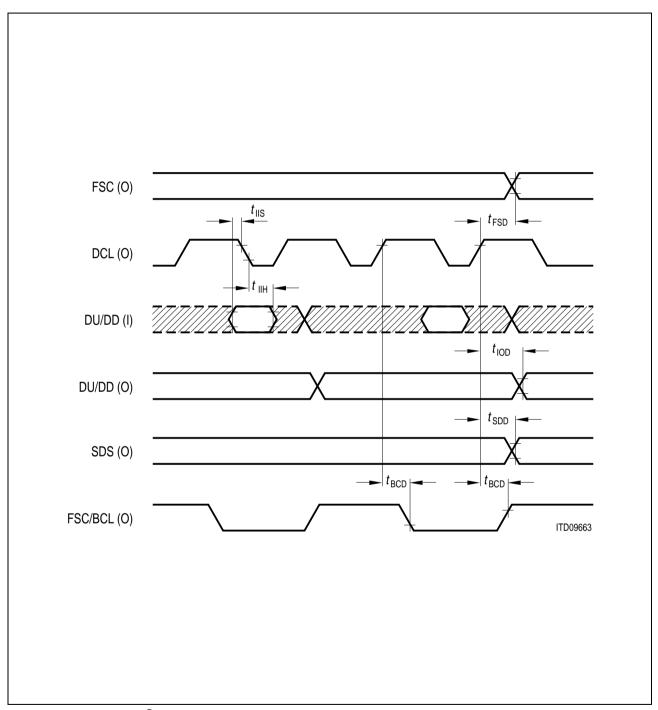
Figure 110 IOM® Timing (TE mode)
