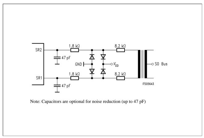
Figure 28 External Circuitry for Symmetrical Receivers
