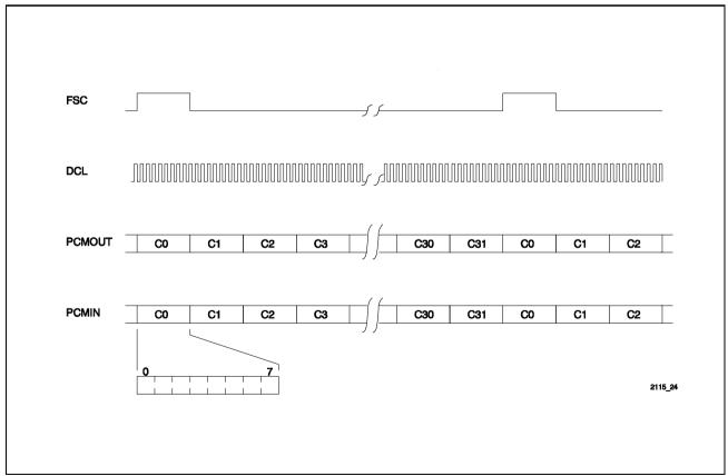
Figure 70 PCM Frame Alignment
