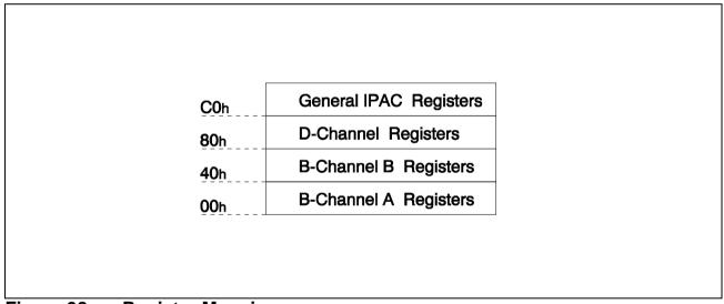
Figure 98 Register Mapping
