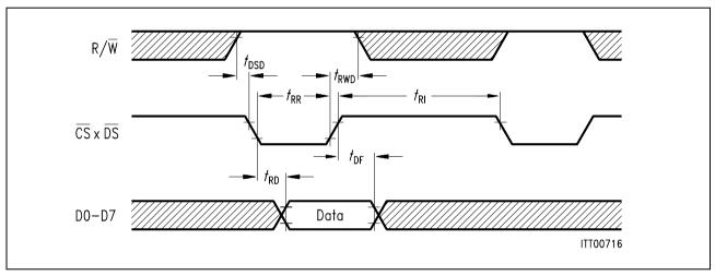
Figure 107 Microprocessor Read Timing
