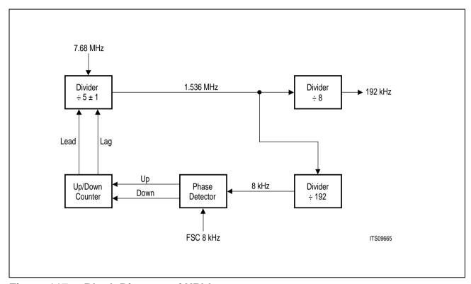
Figure 117 Block Diagram of XPLL
