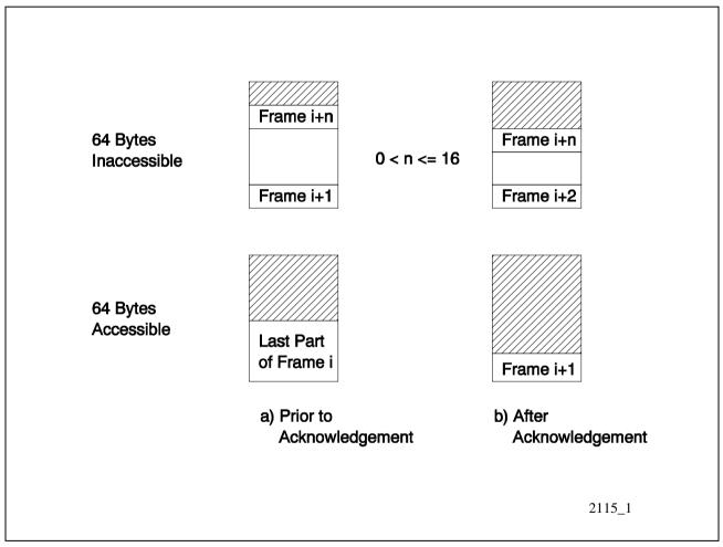
Figure 47 Configuration of RFIFOB (Short Frames)
