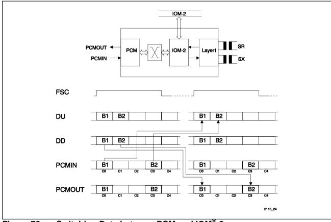
Figure 72 Switching Data between PCM and IOM®-2
