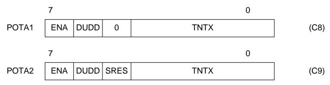
POTA1 refers to the B1-channel and POTA2 to the B2-channel of the IOM channel which is selected by PCFG:CSL2-0.
