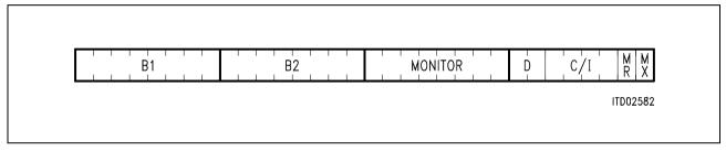
Figure 51 Channel Structure of IOM®-2
