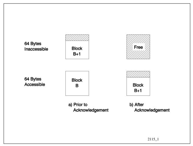
Figure 46 Configuration of RFIFOB (Long Frames)
