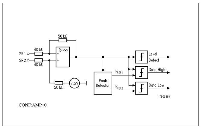
Figure 29 Receiver Circuit
