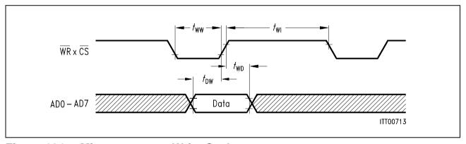
Figure 104 Microprocessor Write Cycle
