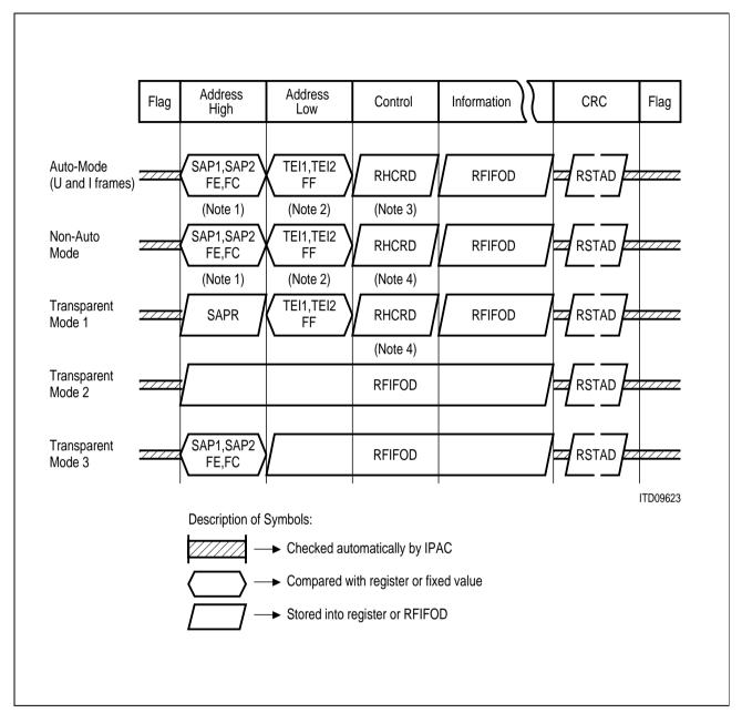
Figure 89 Receive Data Flow
