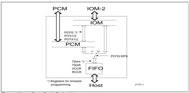
Figure 73 Data Path Switching
