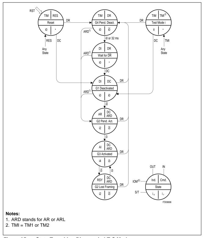
Figure 95 State Transition Diagram in LT-S Mode
