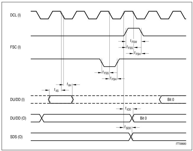
Figure 111 IOM® Timing (LT-S, LT-T mode)
