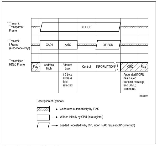
Figure 87 Transmit Data Flow
