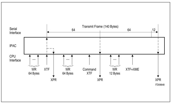
Figure 81 Interrupt Driven Transmission Sequence Example
