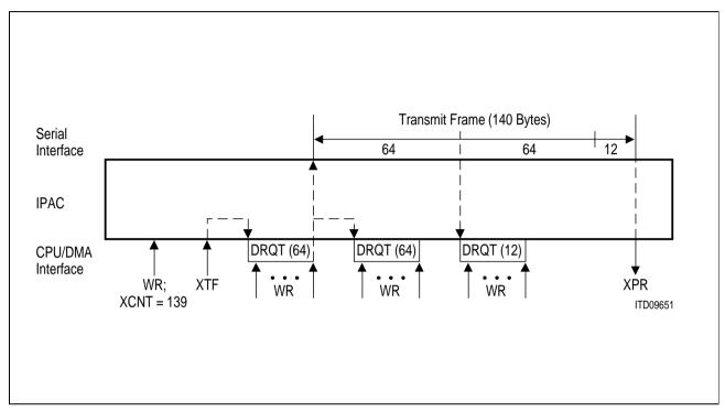
Figure 84 DMA Driven Transmission Sequence Example
