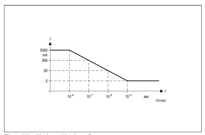
Figure 100 Maximum Line Input Current
