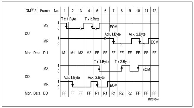
Figure 64 Handshake Protocol with a 2-Byte Monitor Message/Response
