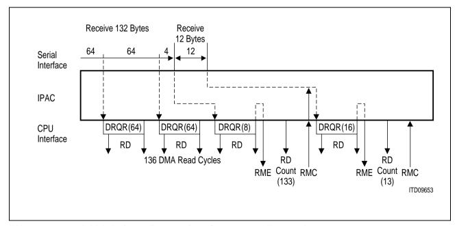
Figure 86 DMA Driven Reception Sequence Example
