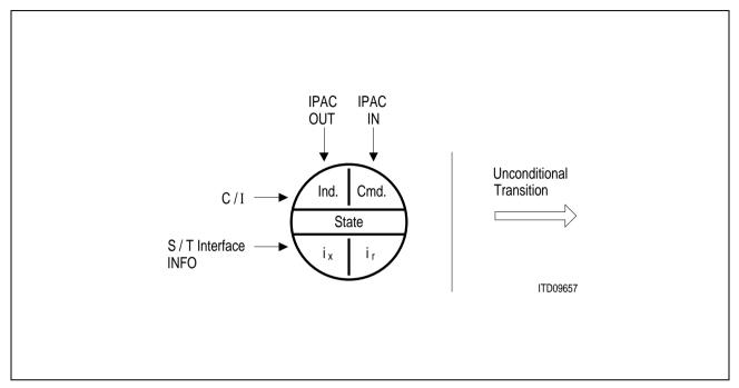
Figure 92 State Diagram Notation
