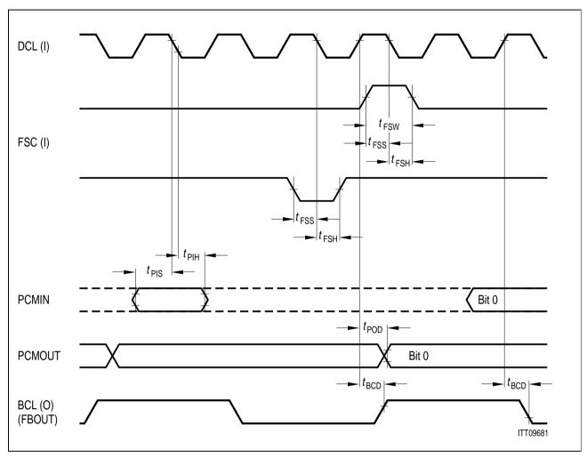
Figure 112 PCM Interface Timing (LT-S, LT-T mode)
