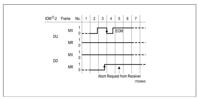
Figure 65 Abortion of Monitor Channel Transmission
