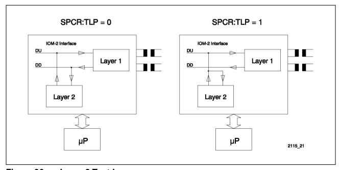
Figure 36 Layer 2 Test Loops
