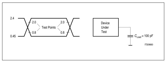
Figure 102 Input/Output Waveform for AC Tests
