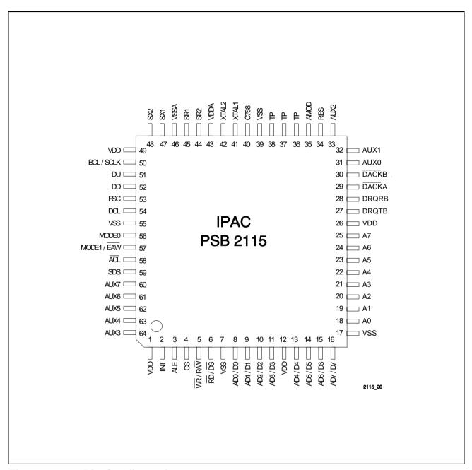
Figure 2 Pin Configuration
