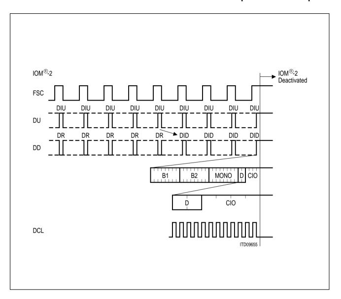
Figure 90 Deactivation of the IOM® Interface
