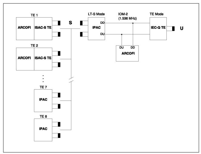
Figure 20 Intelligent NT-Configuration for IOM®-2 Channel Switching
