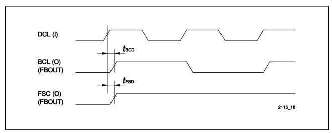
Figure 113 BCL, FSC Output Delay
