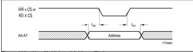
Figure 106 Non-Multiplexed Address Timing
