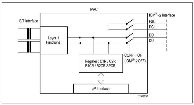
Figure 60 Principle of B/IC Channel Access in IOM®-2 Terminal Mode
