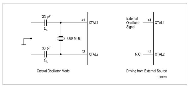
Figure 101 Oscillator Circuits
