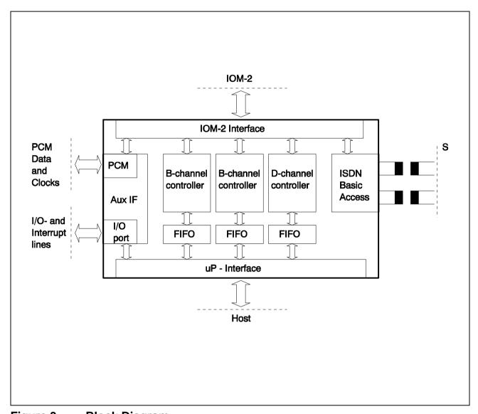
Figure 3 Block Diagram
