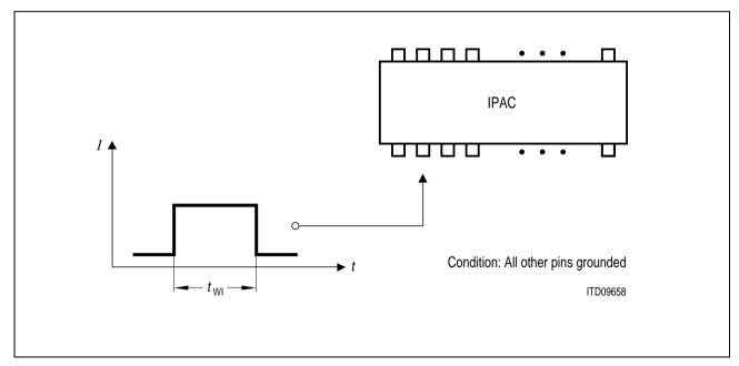
Figure 99 Test Condition for Maximum Input Current
