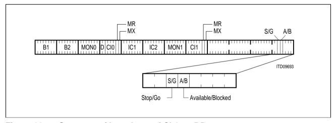
Figure 68 Structure of Last Octet of Ch2 on DD
