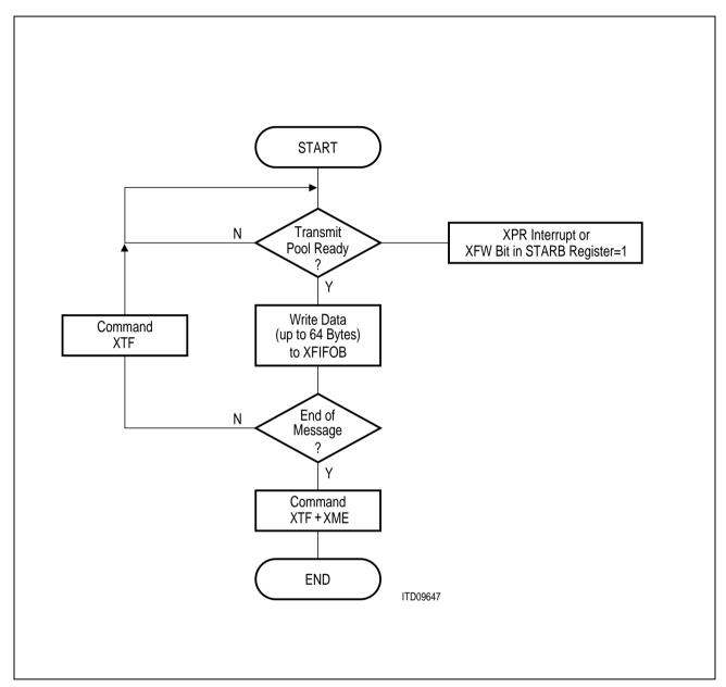
Figure 80 Interrupt Driven Data Transmission (Flow Diagram)
