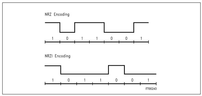
Figure 12 NRZ Encoding/NRZI Encoding
