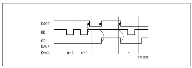
Figure 43 Timing Diagram for DMA-Transfers (slow) Receive (n =  $k \times 64$ )
