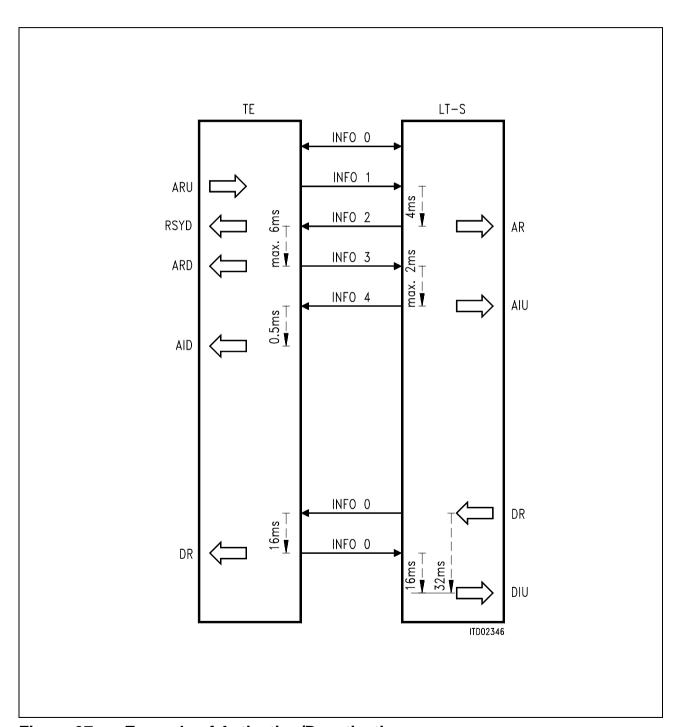
Figure 97 Example of Activation/Deactivation
