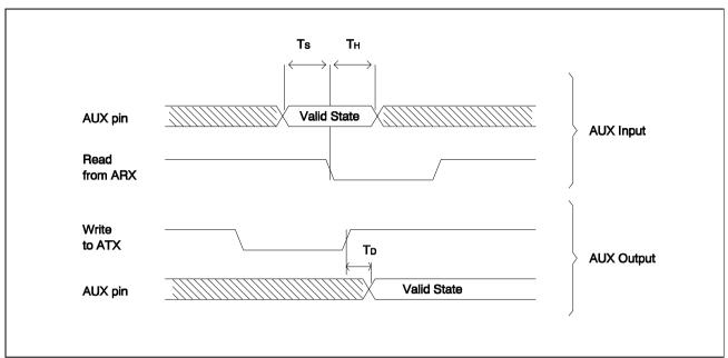
Figure 69 Input/Output Characteristic of AUX Pins
