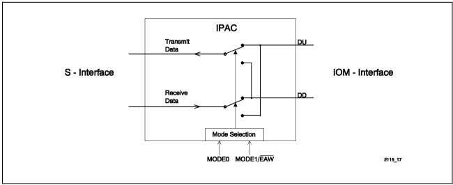
Figure 21 Data Path Switching
