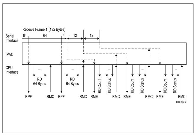
Figure 85 Interrupt Driven Reception Sequence Example
