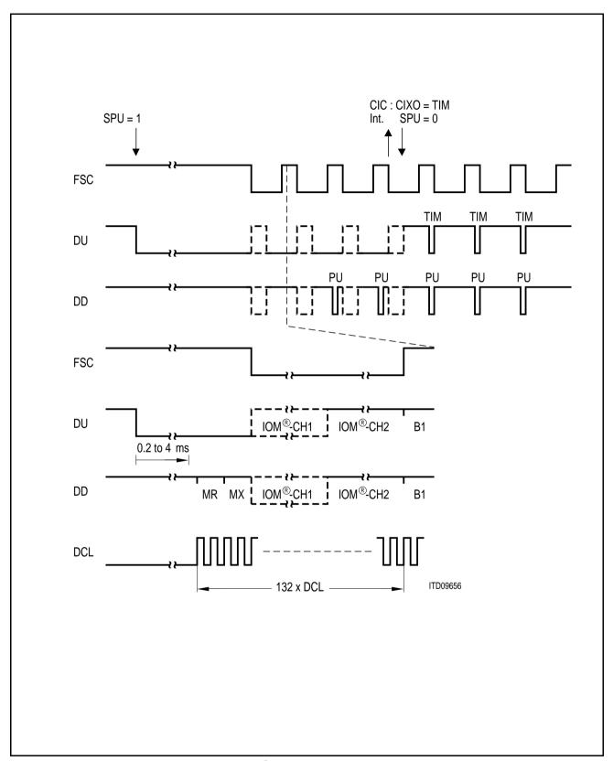
Figure 91 Activation of the IOM® interface
