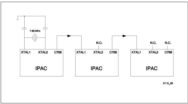
Figure 77 Buffered Oscillator Clock Output
