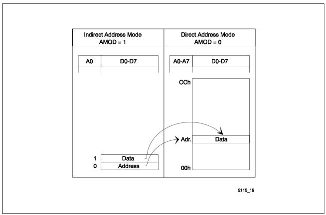
Figure 37 Indirect Register Address Mode
