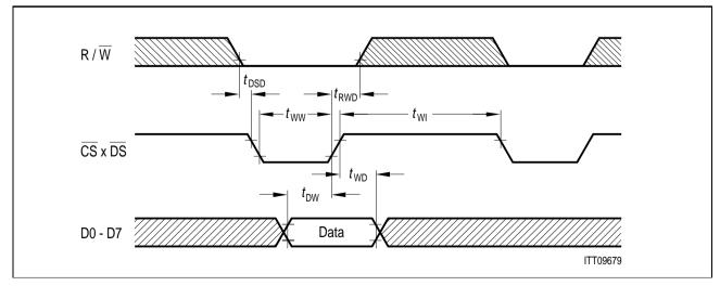
Figure 108 Microprocessor Write Cycle
