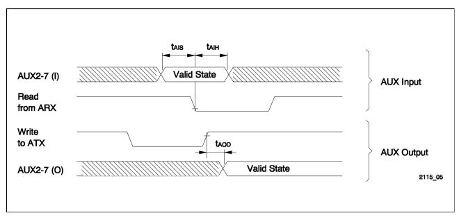
Figure 114 AUX Interface I/O Timing
