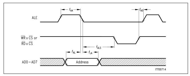
Figure 105 Multiplexed Address Timing
