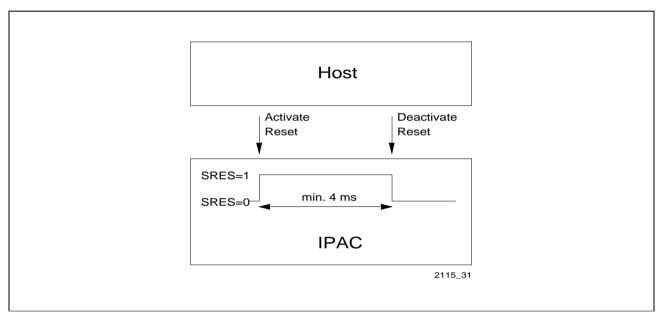
Figure 50 Reset Timing
