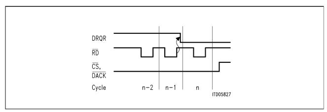
Figure 42 Timing Diagram for DMA-Transfer (fast) Receive (n =  $k \times 64$ )
