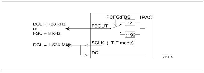
Figure 74 Generation of FSC and BCL in LT-T mode
