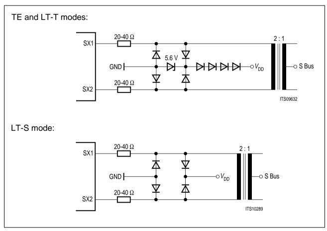
Figure 27 External Circuitry for Transmitters
