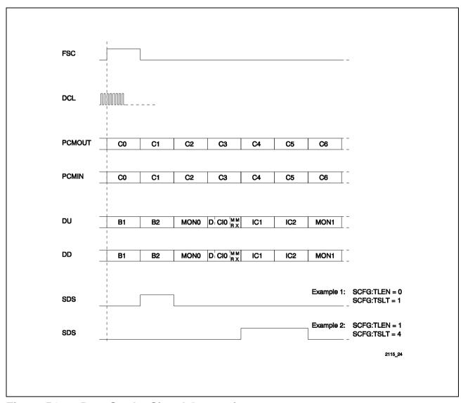
Figure 54 Data Strobe Signal Generation
