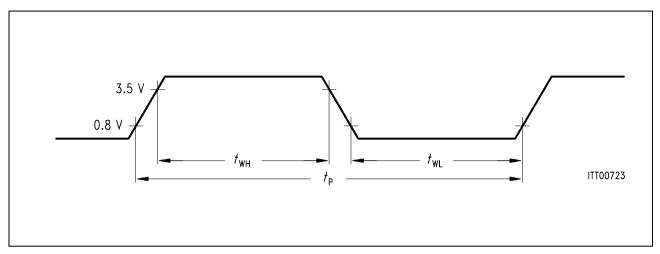
Figure 116 Definition of Clock Period and Width
