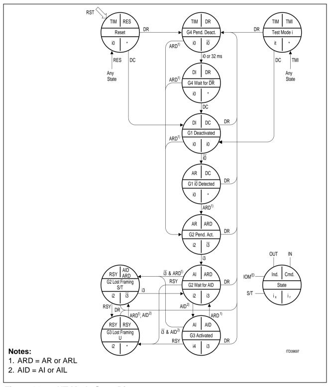
Figure 96 NT Mode State Diagram
