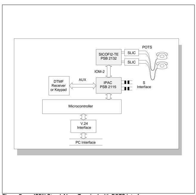
Figure 7 ISDN Stand-Alone Terminal with POTS interface
