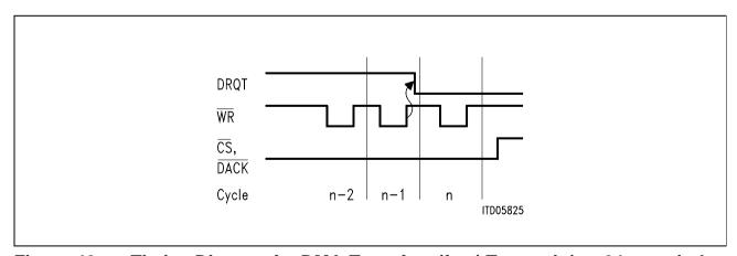
Figure 40 Timing Diagram for DMA-Transfers (fast) Transmit (n < 64, remainder of a long message or n =  $k \times 64$ )
