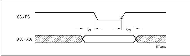
Figure 109 Non-Multiplexed Address Timing
