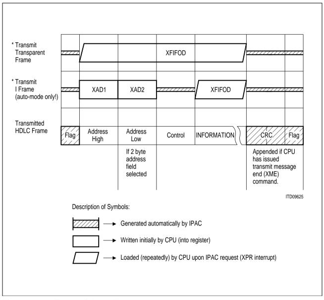
Figure 17 Transmit Data Flow
