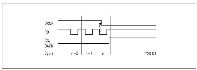
Figure 44 Timing Diagram for DMA-Transfers (slow or fast) Receive (n = 4, 8, 16 or 32)
